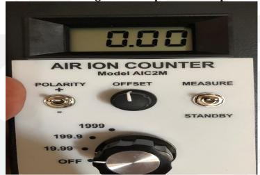
We then turned on the mobile NPBPI unit and read the positive air ION levels at the discharge outlet of the fan and in the space after 5 minutes of run time. The positive air ION levels in the fan discharge air stream read 1,116,000 positive air IONs.
