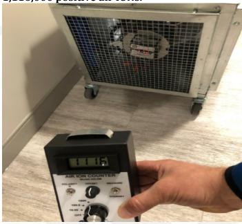
Setting the AIC2M Air ION Counter outside of the air stream on top of the NPBPI module after 5 minutes of operation showed 7,000 Positive air space Ions'
