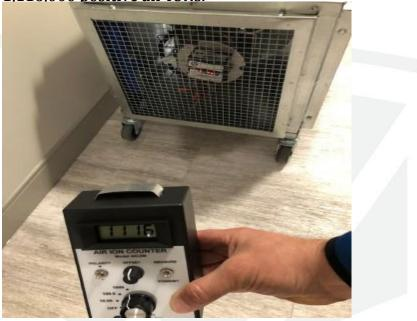
Setting the AIC2M Air ION Counter outside of the air stream on top of the NPBPI module after 5 minutes of operation showed 7,000 Positive air space Ions'
